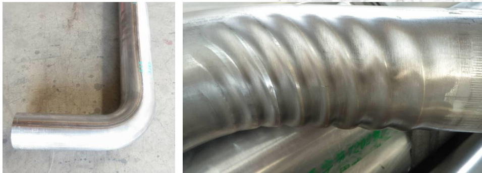
Fig. 2-7: Good pipebend product (left), defective product/wall wrinkles (right)
