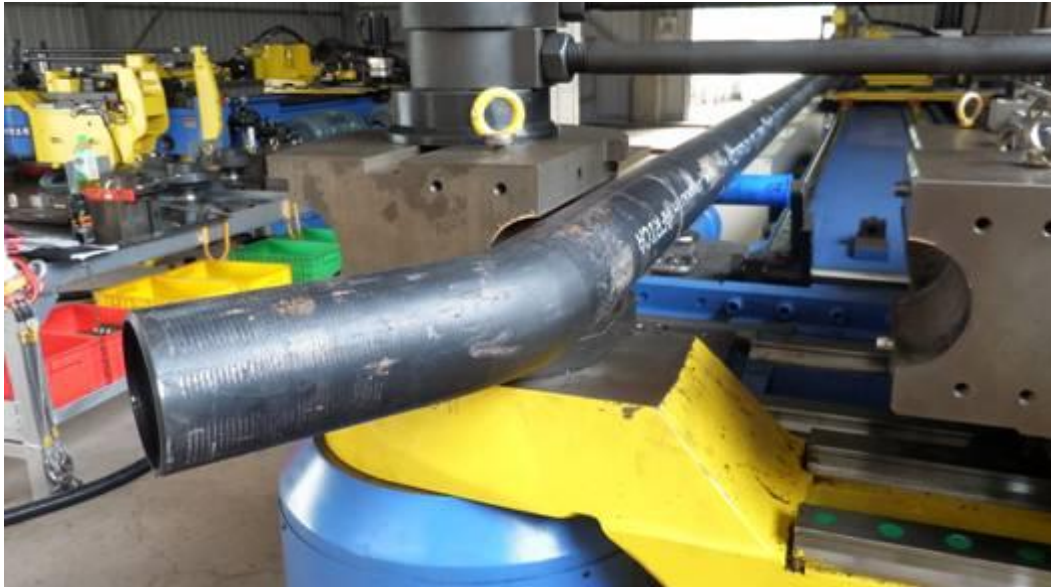
Fig. 2-2: Straight pipe on the digital bending machine for cold bending (The pipe in the photo is 4" _SCH.40S, A106)
