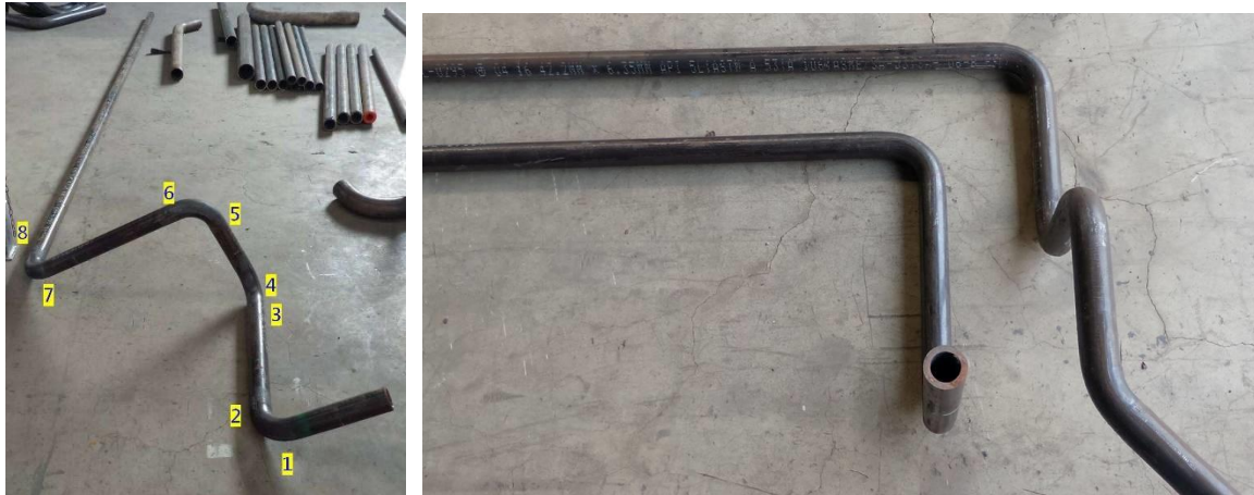
Fig. 2-1: Quick-Bending, this continuous bend can save 8 ring-welds (left), various angle bends (right)
