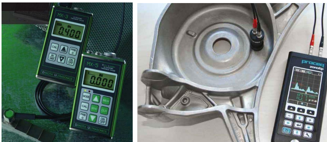
Fig. 3-6: Several Ultrasonic Thickness Gages on the Market (Source: websites of Chuan Hua Precision Co. and YENSTRON Co.)
